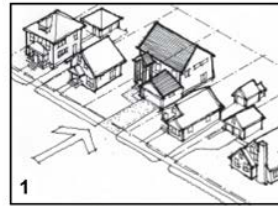
Inappropriate Infill: New house is more massive, disrupts rhythm along street and does not follow existing alignment.
