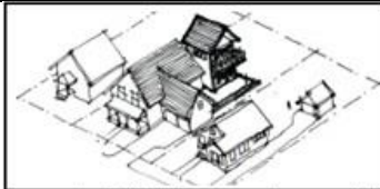
Inappropriate Infill: Tall mass may obstruct sunlight to adjacent yards.
